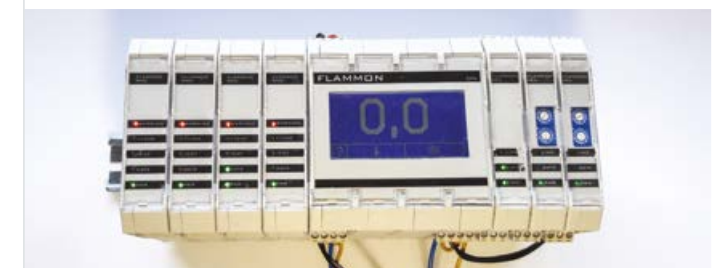
↑ Modules of the processors of the individual optic sensors and central processor
